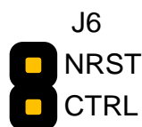
Figure 5-5 – J6: RS500 Reset and USB-UART Control Signal
