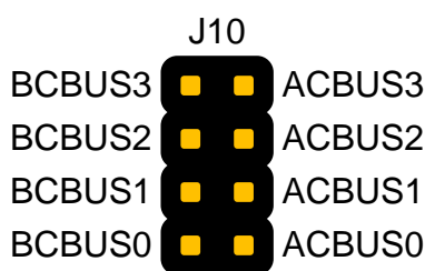
Figure 5-8 – J10: USB-UART ACBUS and BCBUS Outputs
