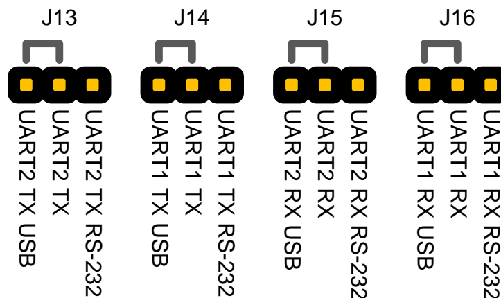
Figure 5-11 – J13-16: UART Selection Jumpers
