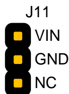
Figure 5-9 – J11: External Voltage Supply VIN
