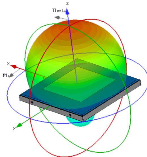
rPad internal antenna radiation pattern
